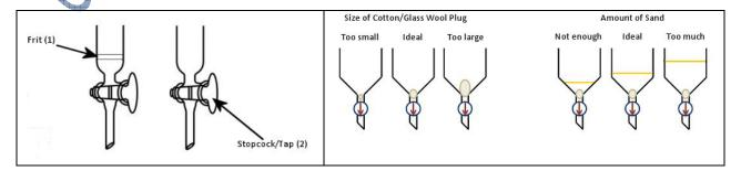
**Figure 2.** Fritted (left) and non-fritted (right) columns.
