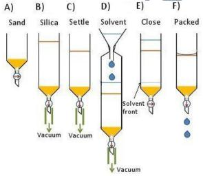
Top Tip: If the column drains faster than expected and the solvent level falls below the top of the stationary phase, add more solvent and gently swirl the column to re-suspend the top few cm of silica. Pipette some solvent down the sides to rinse the column and tap gently to remove any bubbles.
