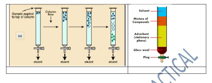
Now put the collecting flask/test tubes at the bottom. The supplied mixture is mixed with dry silica gel and dryed and put in the upper part of the stationary phase. Now solvents from lower % to higher percentage is run. Parallelly you can see the different color bandes in the column. Collect the each band in different test tubes/flasks. Check the TLC of all the testtubes and collect same type of TLC spot in a round bottom flask and dry them separately.
