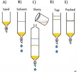
Top Tip: Use hand bellows to increase the pressure in the column and to force the silica to compact. Repeat several times, rinsing the sides of the column in between, to ensure complete packing.
