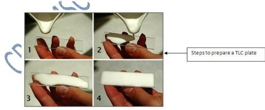
Developing TLC plates using SiO<sub>2</sub> on Glass /Aluminium plate
