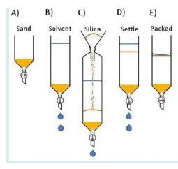
Top Tip: Use rubber vacuum tubing or a cork ring to tap the column and help the silica to settle.
